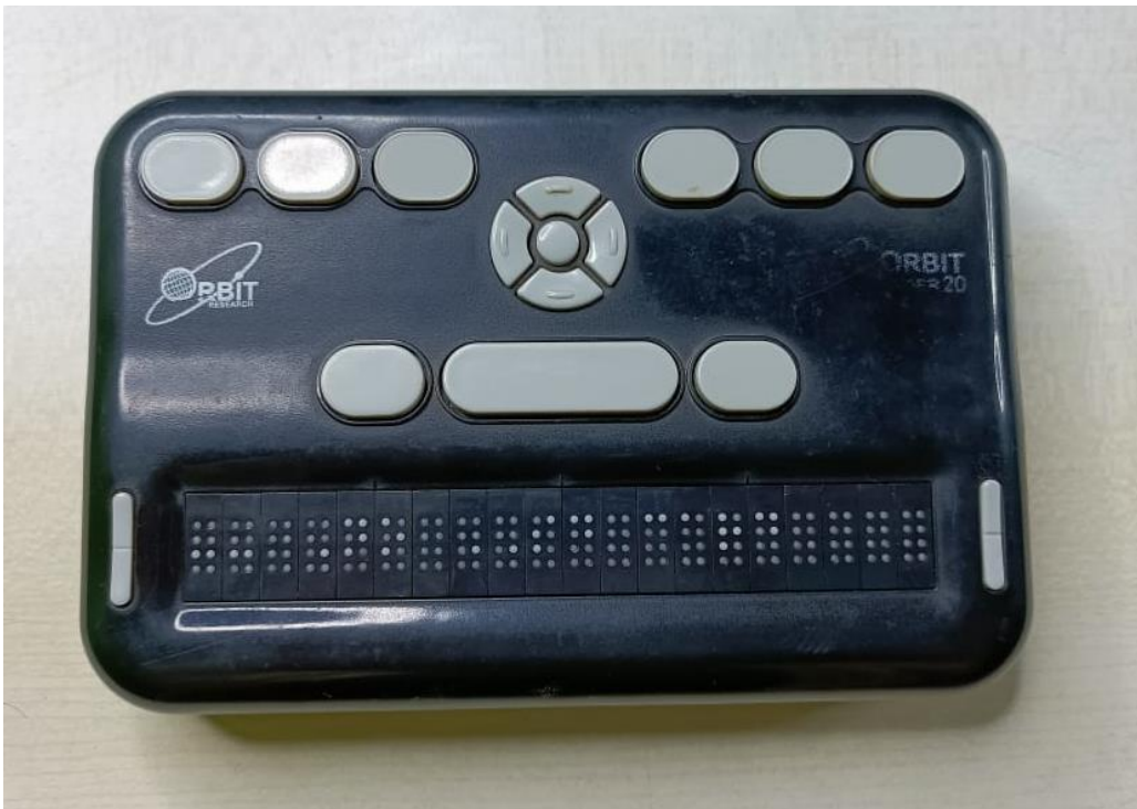
Refreshable Braille display - A vital technology aid for persons with deafblindness
